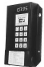
**MODEL 4950PM** - can be mounted through a front panel opening of 2.625 by 4.5 inch cutout. It features a tactile type of keypad 1-9 and # with an overlay. Two SPST-NO contacts rated for 20 amperes can be individually programmed. Time of day is maintained in a smart timepiece circuit that will keep the time running for up to 5 days during a power failure without the use of external batteries.
