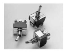
The H-Series toggle switches are heavyduty, high voltage, high amperage, threepole switches. These switches have a contact slow-make, slow-break mechanism, are AC rated to 600V, and are available in a wide range of ratings, circuits, terminations and bushing/toggle configurations.
