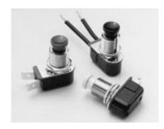
The P27-Series pushbutton switches are single pole, AC/DC rated switches suitable for shallow back panel applications. These switches are momentary action with a medium actuation force (26 oz. typical). The P27-Series switch is equipped with a slowmake, slow-break contact mechanism, rated at 6 amps with a nylon concave pushbutton.
