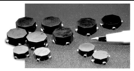
ECONO-PACs and OCTA-PACs are versatile surface mount magnetic devices that can be used in design applications as single inductors, coupled inductors, or 1:1 transformers providing isolation between the two windings. OCTA-PACs are designed around Kool-Mu<sup>™</sup> material which allows maximum power density with lowest core losses. ECONO-PACs, lower cost versions of OCTA-PACs incorporating powdered iron cores, deliver frequency responses to several megaHertz.
