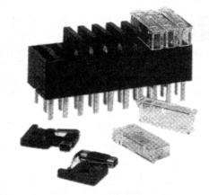
Designed for use with HLT, HLS and PCT fuseholders. Voltage Rating: 60V DC, 125 VAC. Interrupting Rating: 450A at 60 VDC, 300Å at 125 VAC. Thermoplastic body meets UL 94V-0 Flammability Test. Beryllium copper terminals. UL Recognized, Guide JFHR2, File E56412. Packaged 10/ctn.
