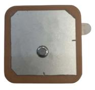
GPS, GLONASS, Galileo, & BeiDou Standards Dimensions: 25mm x 25mm x 4mm Frequency: 1575.42/1602/1608MHz
