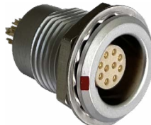
MMI-M1FSXXXS Female, Panel Mount Size 1, Solder Cup
