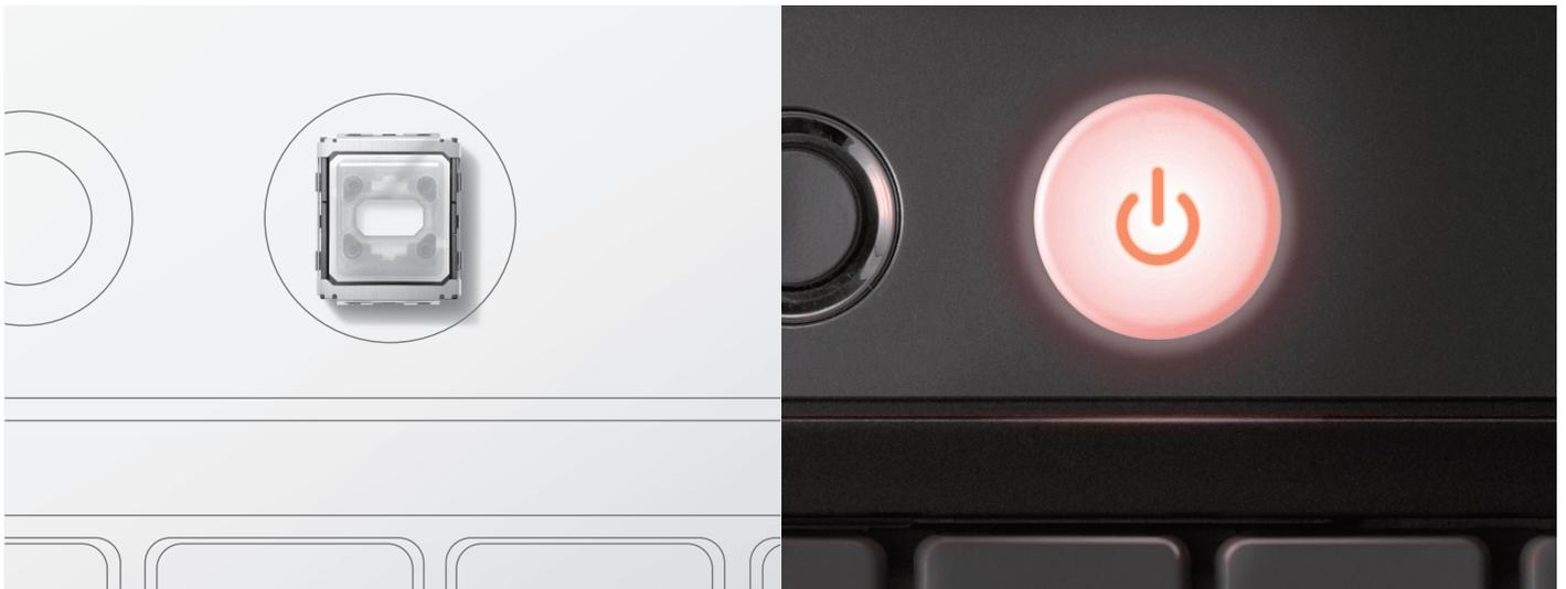
**Original mechanical structure realized soft clicking feel and long travel of 1.1mm.**
