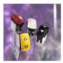
The KR Series is available with solder lug/quick-connect and screw terminals and with or without a plastic barrier between terminals. Up to 10 terminals are offered to allow for multiple electrical and illumination possibilities. Materials include silver contacts and UL94-VO rated engineering plastics. The switch is designed to be mounted into a 1.450" x .830" panel cut-out.
