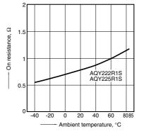
2.-(2) On resistance vs. ambient temperature characteristics
