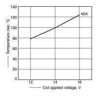
1.-(1) Coil temperature rise (85°C 185°F) Sample: ACW212, 3pcs Point measured: Inside the coil Contact carrying current: 45A Ambient temperature: 85°C 185°F
