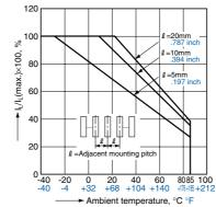
3. On resistance vs. ambient temperature characteristics
