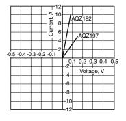
10. Leakage current vs. load voltage characteristics
