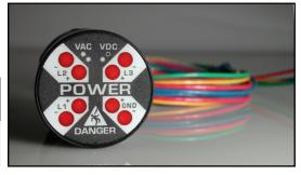
NOTE: For 3-Phase Wye applications, it is normal for the "GND" indicators not to flash unless phase is lost.
