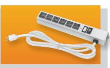
voltage. Prevents equipment damage, lost or distorted data. Maximum surge current is 13000 amps, response time is < 5ns., 15 amp thermal type circuit breaker with reset. 14 gauge, 3 wire, 6 foot power cord, all components UL approved.
