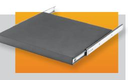
Sliding shelves, available in ventilated and non-ventilated versions, fit 19" and 24" wide panel spaces and all cabinet rack depths. Shelves are 16-gauge steel and flanged on all four sides for added support. Universal mounting brackets allow flexibility in mounting. Shelves allow sufficient room in rear for cables and power outlet strips. Requires two pairs of panel mounting rails per cabinet rack. **Finish:** Smooth Black
