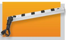
wires. Strips snap into adjustable mounting clips. Grounding type 15 amp., 125 volt receptacles, 15 amp thermal-type circuit breaker with reset. 14 gauge, 3 wire, 6 foot power cord. All components UL approved.
