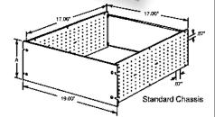
Side Panel mounting holes are punched on .87<sup>"</sup> grid to allow total flexibility in mounting of components. Rear Panel is fully adjustable from front to rear. Standard 19.00<sup>"</sup> Front Panels feature "Surface Shield" protection, which provides surface for laying out drilling and punching positions.
