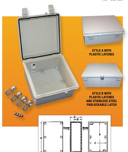
⊢ H+ G → These gasketed all-plastic enclosures have been designed meet NEMA 1, 2, 4, 4X, 12, 13 and IEC529-IP66 requirements, which allows them to be used in many wet, dirty and/or corrosive environments.
