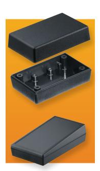
Styles A & B have squared corners, provisions for mounting horizontal and vertical PCBs, and four non-skid feet. ABS plastic, UL94-HB flammability rating. Available in black (-B) or gray (-G).
