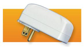
Enclosure for devices mounted in a standard 125VAC power plug. Includes integral 125 VAC plug with through-hole solder terminals inside and external mounting flange in base. Durable ABS plastic has UL94V-0 flammability rating. Internal PCB mounting bosses in base. Cover is securely attached to the base with four matched screws.
