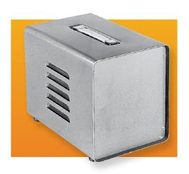
.05" aluminum. Front panel recessed .50" and fits contour of cabinet. Louvered sides. Welded back has opening. Four plastic feet furnished.
