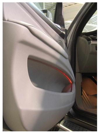
concept in front and rear door panels. The longitudinal light guides placed in the door storages highlight the car's interior luxury, materials and craftsmanship. It also allows a better seek of elements stored in the door: pens, maps, wallet, flashlight...
