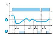
Monitoring a level, filling function, activation time
