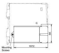
When a PS9Z-6R1F is installed on PS6R
