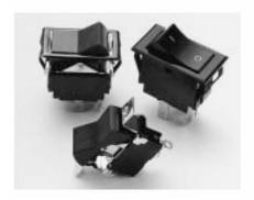
The TI-Series Tippette rocker switches are available in single pole (TIL), double pole (TIG), three pole (TIH) and four pole (TII) versions. These switches are available with nylon snap-in or screwtype mounting brackets, are AC rated to 20 amps and suitable for low voltage DC applications. Multiple actuator options and colors are available, and many circuits have international approvals.
