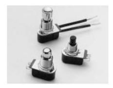
The P26-Series pushbutton switches are single pole, AC rated for 8 amps at 125 VAC and suitable for shallow back panel applications. These switches are momentary action with a medium actuation force (13 oz. typical). The P26-Series switch is equipped with a slowmake, slow-break contact mechanism.
