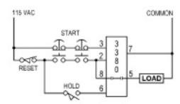
Note: The Reset and Hold switches shown in the above wiring diagrams are optional and are not required for all applications.
