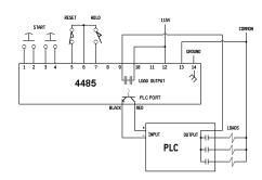
Note: The Reset & Hold switches shown in the above wiring diagrams are optional and are not required for all applications.
