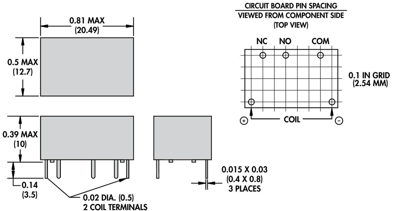
DRAWING AND PIN SPACING ENLARGED TO 200% OF ACTUAL SIZE
