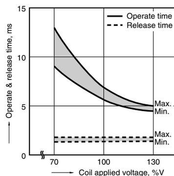
5-2. Operate & release time (with diode)
