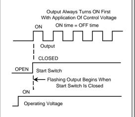
The timing diagram shown below is for an application that requires the load circuit to be ON for 20 milliseconds and OFF for 20 milliseconds. (Remember - the ON and OFF times will essentially be equal due to the 50% duty cycle specification inherent in the model 4280)
