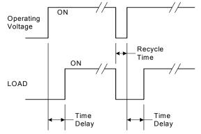
Load turns ON after time delay, remove power for Recycle Time to reset timer
