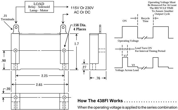
When the operating voltage is applied to the series combination of the 438FI and the load circuit, the 438FI turns ON, and the
