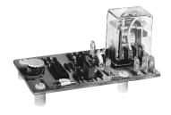
The model 4606, open board flasher, combines digital timing techniques with 10 ampere output contacts to form a flasher that is available in either AC or DC operating voltages. The model 4606 is available in fixed flash rates from 1 to 250 FPM, and adjustable models in two ranges covering 1 to 250 FPM. The model 4606 is essentially a 50% duty cycle flasher. This means that the energize time and the de-energize times are essentially of equal timing period.
