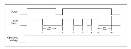
the *Output* turns ON, energizing the load. The *Initiate Switch* opens and closes at times #5, 6, 7, and 8, but recloses before the end of the timing period keeping the *Output* ON and the load energized. At time #9 the Initiate Switch opens and remains open longer than the timing period causing the Output to turn OFF at time #10.
