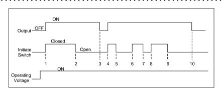
time #4, the *Initiate Switch* closes and the *Output* turns ON, energizing the load. The *Initiate Switch* opens and closes at times #5, 6, 7, and 8, but re-closes before the end of the timing period keeping the *Output* ON and the load energized. At time #9 the Initiate Switch opens and remains open longer than the timing period causing the Output to turn OFF at time #10.
