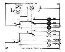
NOTE: Minimum sw open time: 100 ms. Minimum sw close time: 20 ms. Output Pulse length — approx. 50 ms.
