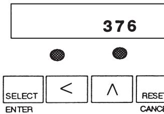
After one of these options is displayed for a second, the value for this option is automatically displayed. Once the option value is displayed, pressing the < key will move one digit to the left and the ^ key will increment the value by one. Then the
