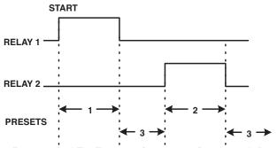
For a standard Flip-Flop timer / counter set Preset 3 to "0".
