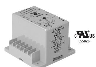
The **AC 2020 Compressor Protector** provides multimode **time delays**, **reset** selections and a **memory capability** which indicates using LED's, the last fault condition. This offers not only protection for the compressor in adverse electrical conditions but also a method to readily determine the type of fault occurrence.
