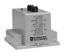
The **CDO Series** is used to detect **OVER CURRENT** conditions. The internal relay energizes (Pick-up) when the monitored current exceeds the preset trip point for longer than the adjustable time delay. The delay is incorporated to prevent nuisance tripping caused by inrush currents. The CDO has an automatic reset feature. The internal relay de-energizes (Drop-out) when the current drops 5% below the preset trip for longer than 0.2 seconds.
