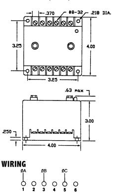
The SLH Series is designed to protect equipment against PHASE LOSS (single phasing), UNDER VOLTAGE (brown outs), and PHASE REVERSAL (improper sequence).
