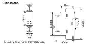
Symmetrical 35mm Din Rail (EN50022) Mounting
