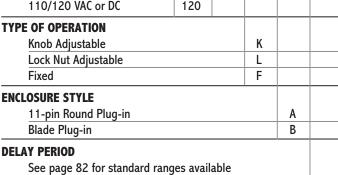
Example: TDJ-120-ALA-300—Delay on Operate/Delay on Release, 120 Volts AC or DC, lock nut adjustable from 3 to 300 seconds, 11-pin octal plug-in, UL recognized.
