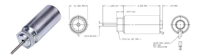
Solenoid shown energized with plunger fully seated Supplied with hex nut shipped loose Spring kits available (consult factory)
