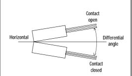
These switches operate when tilted from the horizontal position. The switch movement required to cause contact change (example off to on) is called the differential angle.
