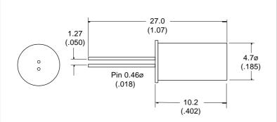
Differential angle varies if pins are aligned vertically (as drawn) or horizontally
