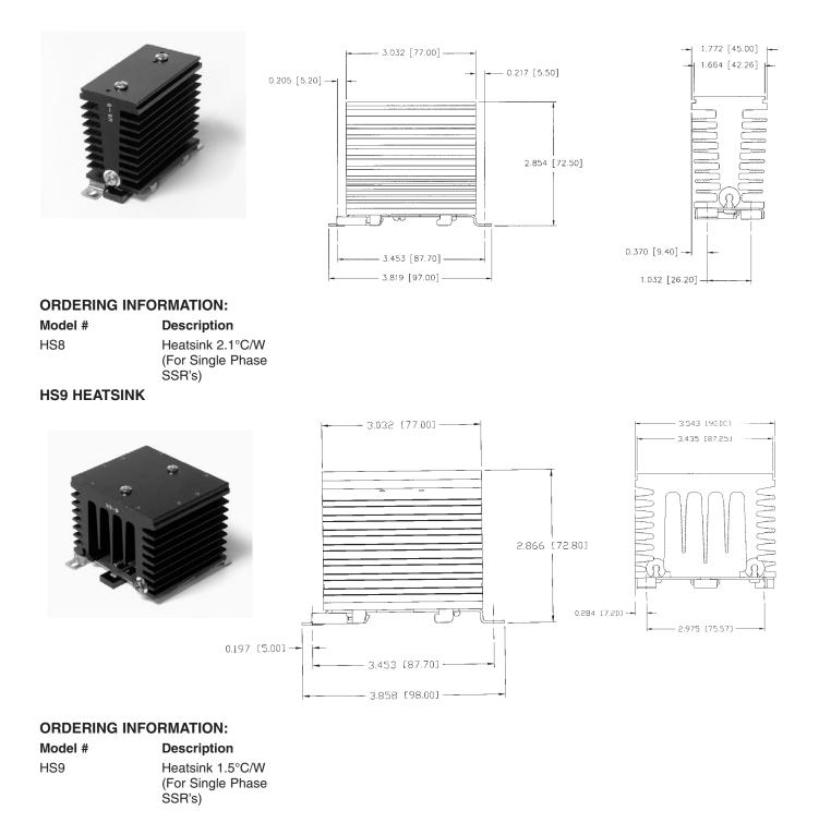
DIMENSIONS: inches (mm) TOLERANCES: ±0.02 inches MATERIAL: AISI 6063-T5 Aluminum FINISH: Black Anodized
