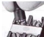
Insulated phosphor-bronze connector clamps to over head of No. 10-32 terminal screws. Test lead and test jumper are constructed from 6' length of No. 14AWG wire. Test lead is fitted with connector at one end only, while test jumper has connectors at both ends. Connectors eliminate use of alligator clips and are rated 50 amps intermittently at 15 amps continuously.
