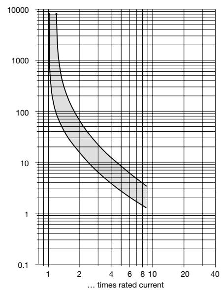
The time/current characteristic curve depends on the ambient temperature prevailing. In order to eliminate nuisance tripping, please multiply the circuit breaker current ratings by the derating factor shown below. See also section 9 – Technical information.
