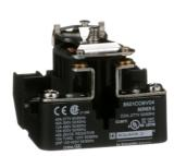
Power Relay, Type C, 2.0 HP, 30A resistive at 300 VAC, SPST, 1 normally open contact, 277 VAC coil
