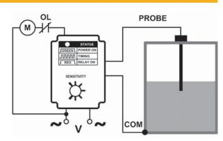
If the container is non-conductive or insulated, an additional probe must be installed as the COM connection where it will always be submerged.
