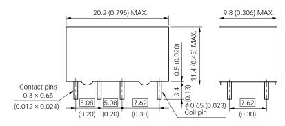
(Note) The tolerance is  $\pm 0.2$  (0.008) unless otherwise specified. The dimension in the box shows basic size.
